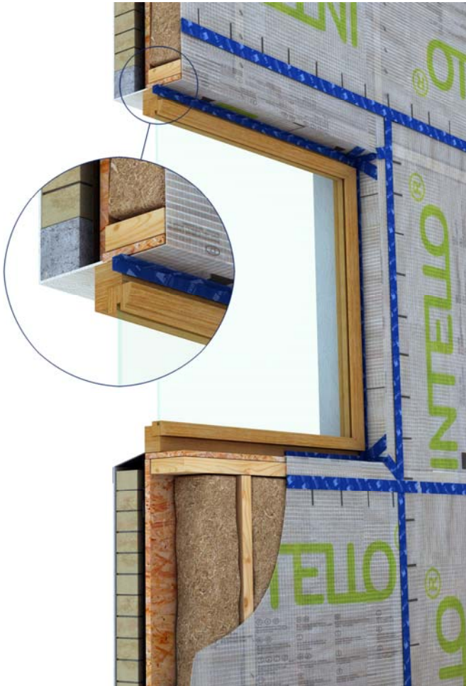
Figure 2: Window Detail sealed with TESCON PROFIL
