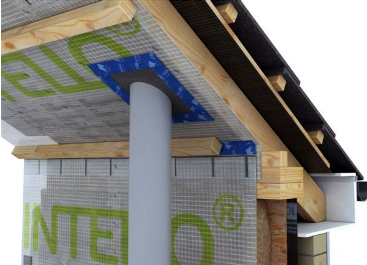
Figure 4: Roof Detail with Pipe Grummet
