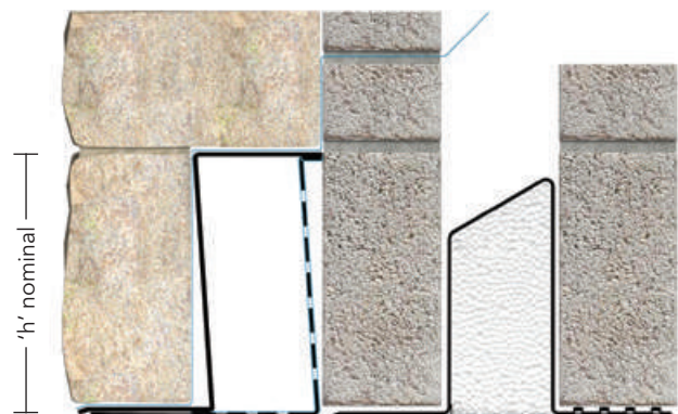
BOX/K-200 lintel shown with optional feature plate.
