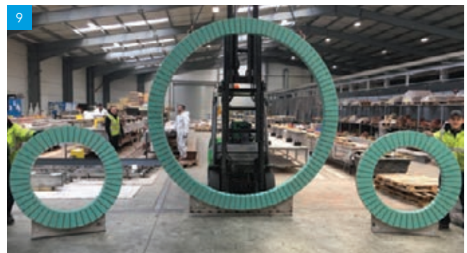
9 Bullseye Arches with glazed bricks
