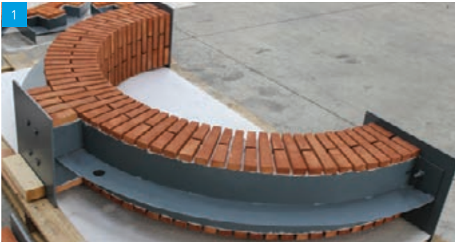
1 Segmental Arch with Keystone in production
